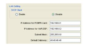
After Quick Setup is completed, if the IP addressing information was not changed and a V-IPEXT card was installed during setup, the IP-PT registration screen is displayed. For information on registering IP-PTs to the PBX, see **3.15** [1-1] Slot—Port Property - Virtual IP Extension. You may now begin programming the PBX.
